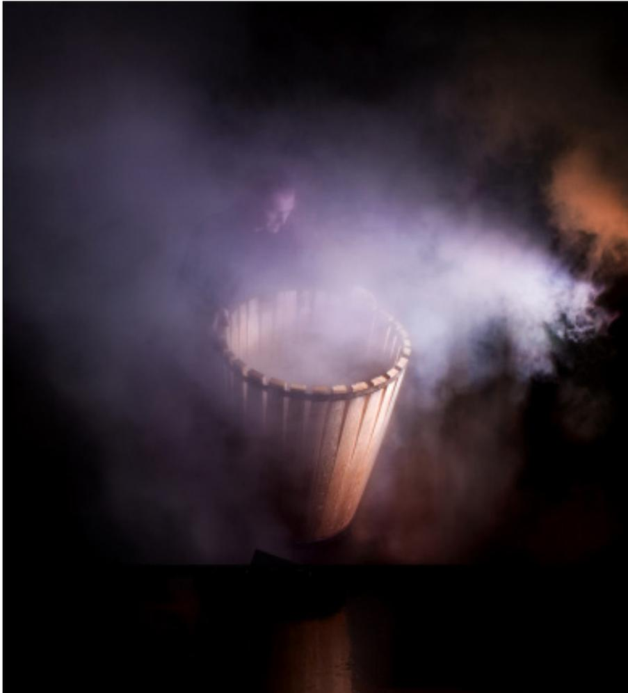
To shape the barrels Tonnellerie Berthomieu uses a unique technique of bending using steam.
